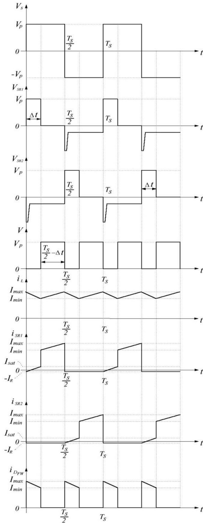
Fig. 3. Waveforms of a push-pull MagAmp regulator
