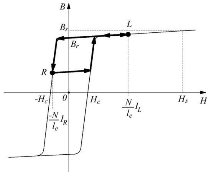
Fig. 1. MagAmp switching trajectory in B-H plain
