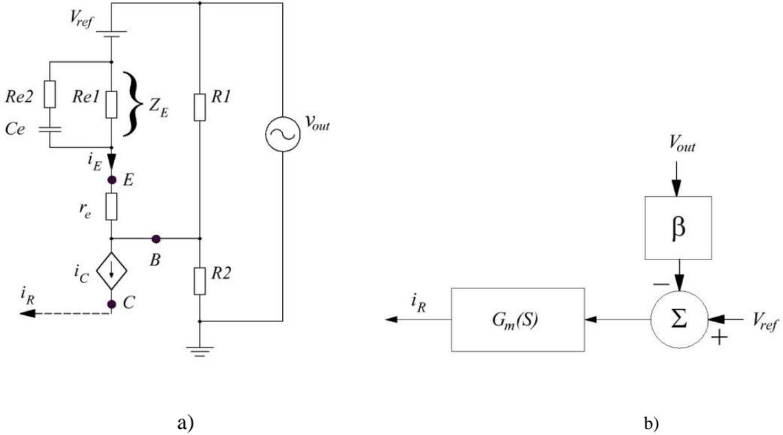
Fig. 6. MagAmp controller equivalent circuit a) and its small signal model b)
