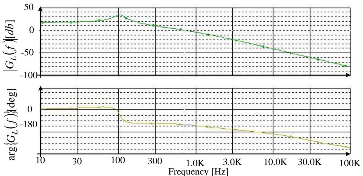
Fig. 8. Simulation results: overall frequency response of MagAmp post-regulator loop-gain  $G_L(f)$ . Top trace: Magnitude [db]; bottom trace: Phase [deg]
