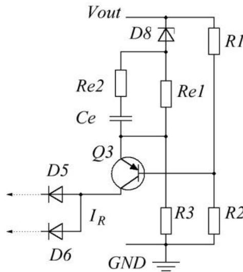
Fig. 4. Control circuit of MagAmp post-regulator
