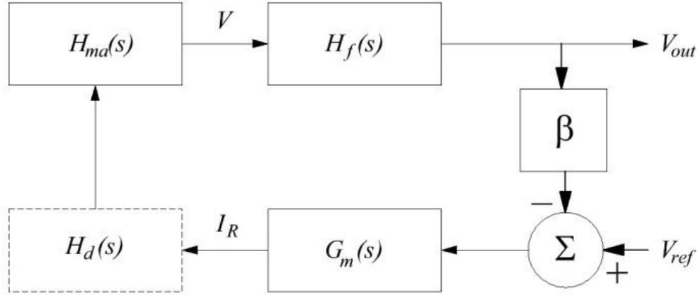
Fig. 5. Average model of MagAmp control loop
