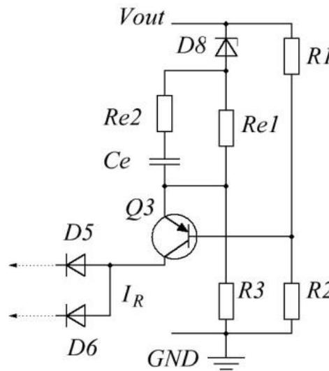
Fig. 4. Control circuit of MagAmp post-regulator
