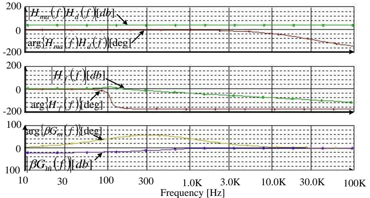
Fig. 7. Simulation results: frequency response of MagAmp post-regulator control loop components. Top trace: MagAmp frequency response including the delay,  $H_{ma}(f)H_d(f)$ ; middle trace: output filter frequency response,  $H_f(f)$ ; bottom trace: control circuit frequency response  $\beta G_m(f)$ .
