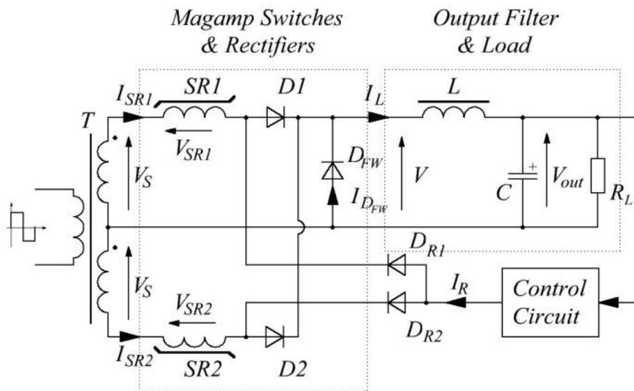
Fig. 2. Push-pull MagAmp regulator circuit
