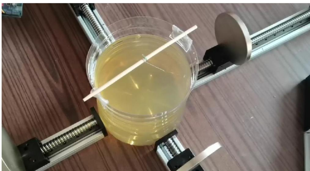
Figure 9 –The small permanent magnet moves along the inner wall of the container towards a second large permanent magnet
