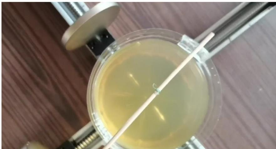
Figure 12 – The small permanent magnet moves along the inner wall of the container towards the fourth large permanent magnet
