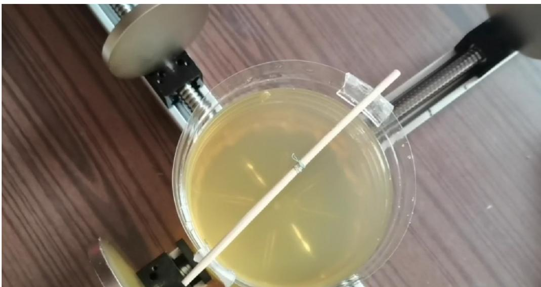
Figure 11- The small permanent magnet stays near the third large permanent magnet
