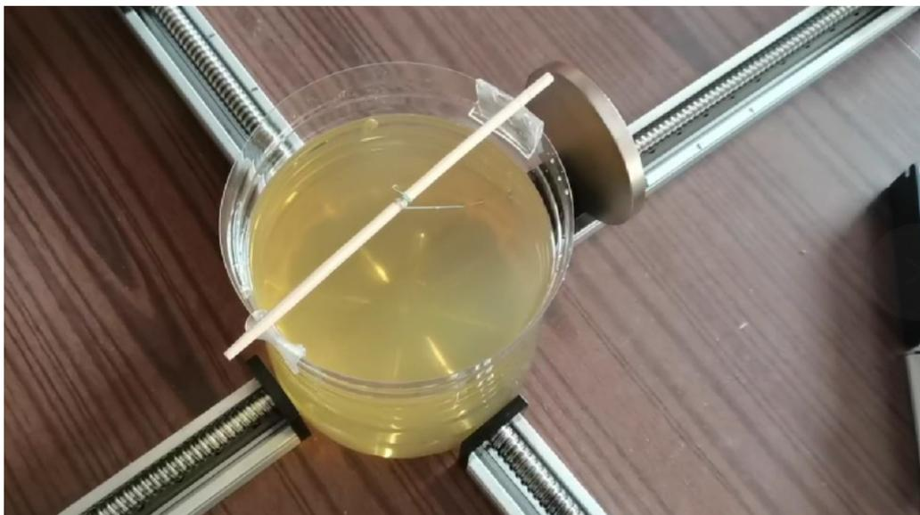
Figure 8 – The small permanent magnet moves towards the first large permanent magnet
